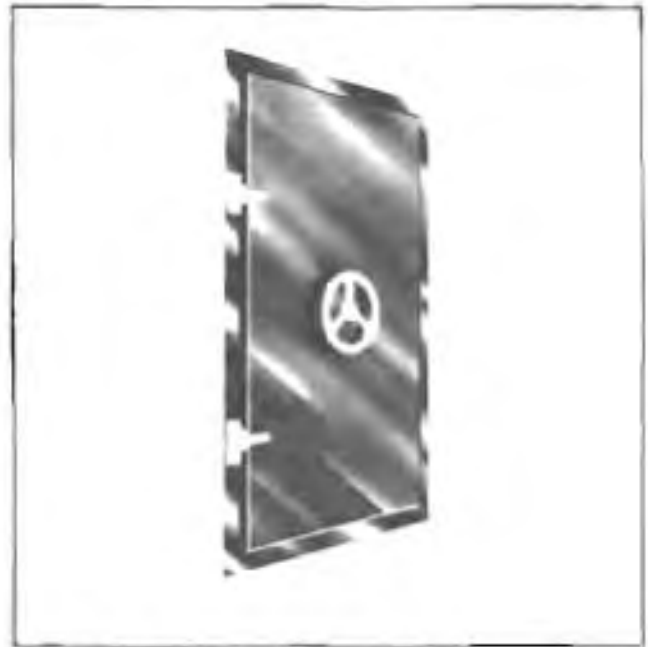
Figure I-11. Watertight Hinged Door
