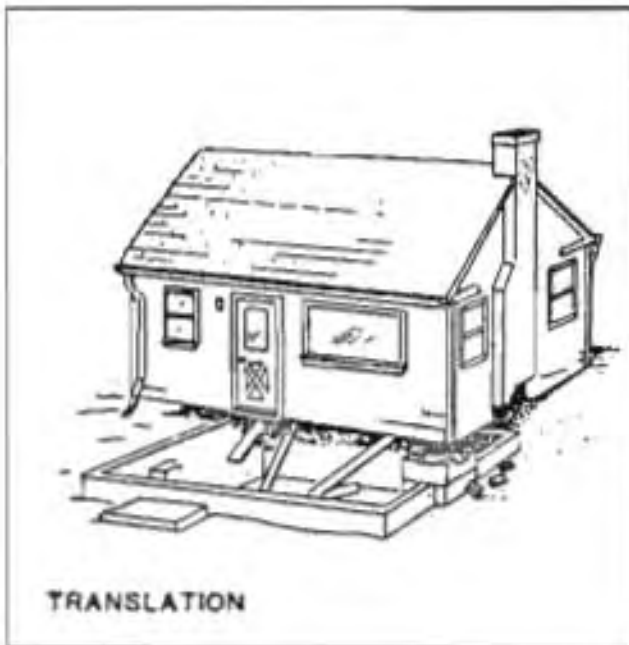
Figure D-1. (cont.) Effects of Floodwater
