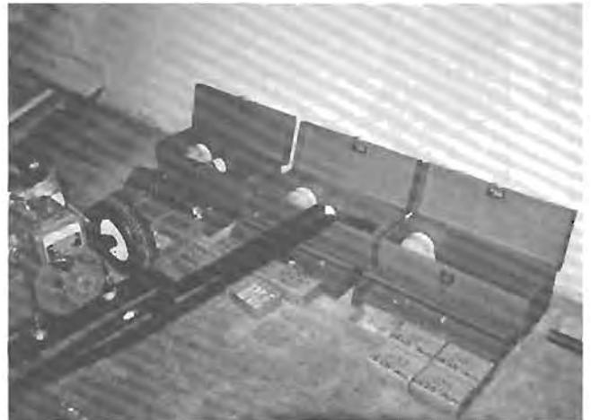
Tools, parts, and portable gas powered pumps required to install flood shields and remove any seepage that may occur.
