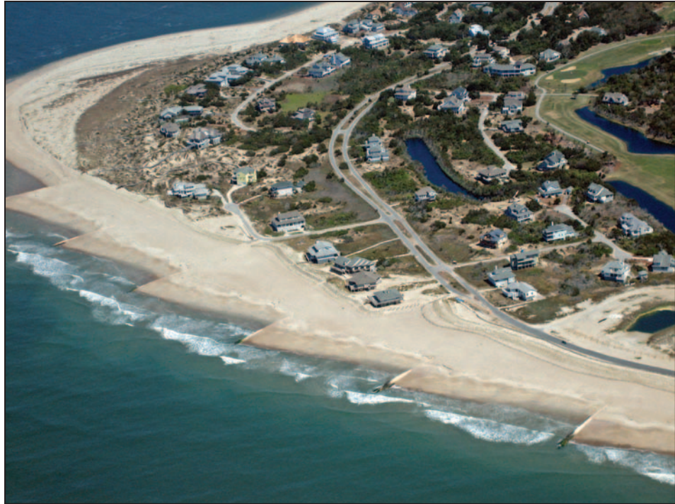
Figure 4-5. Groins were installed in an attempt to stop erosion (note narrower beaches downdrift of groins, as shown also in Figure 2-12)
